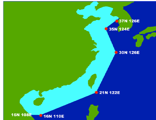
Figure 1. Schematic diagram of the definition of TC landing. The TCs entering the area to the northwest of the polyline along the coast of China are considered as landing TCs.
